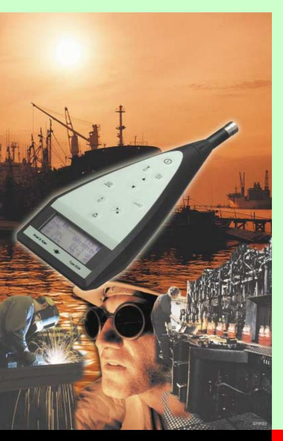
Type 2239 A is a Type 1 sound level meter that is designed to be quick and easy to use when making environmental noise and occupational health related measurements. A large LCD screen displays measurements and includes a quasi-analog bar showing the current sound pressure level. The instrument has two parallel, independently weighted detectors that enable it to display RMS and Peak readings simultaneously.
